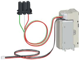
In MasterPact MTZ devices, diagnostic and/or communicating voltage releases are continuously supervised by the control unit when they are declared in EcoStruxure Power Commission software. If a breakdown or power outage occurs, or the recommended number of operations is reached, an alarm is generated to take action for replacement.
